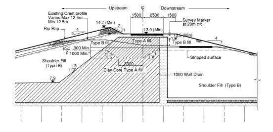
Figure 7 Final Dam Crest Detail
